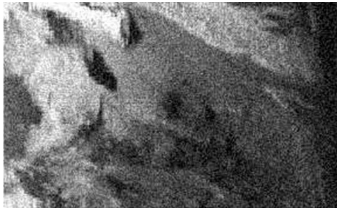
Figure 4.20. Example of speckle (high-frequency noise) in a sonar image.
