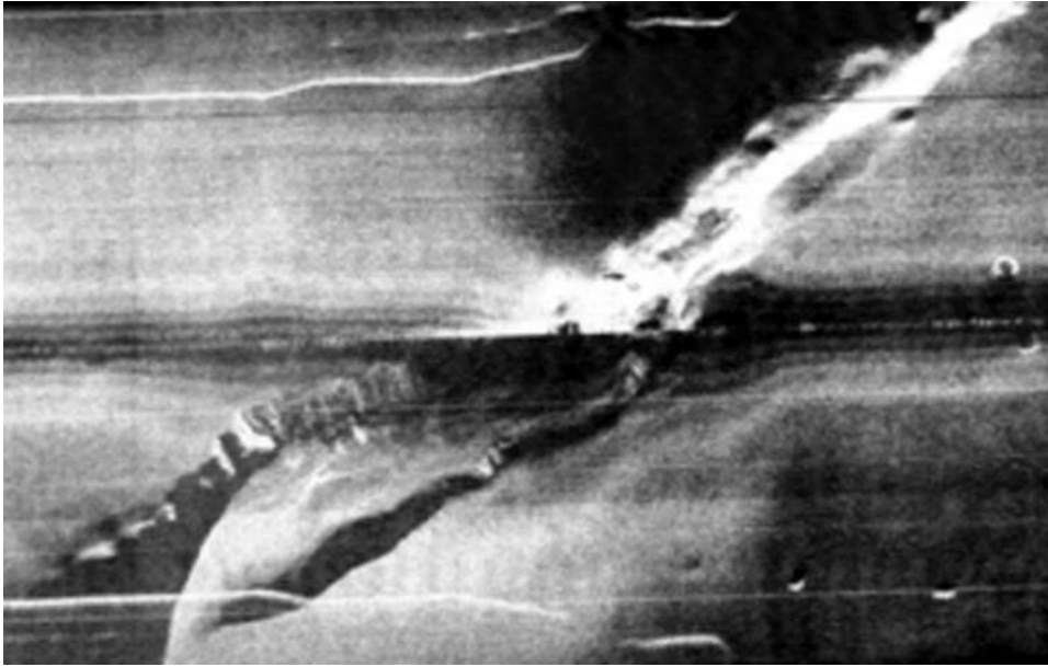
Figure 7.18. Uncorrected MAK-1 record of a fault scarp in the Mediterranean Sea. The image corresponds to a full MAK-1 swath and is 2 km wide (from Beijdorff et al. , 1994; © UNESCO).
