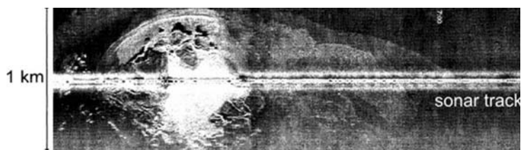
Figure 7.25. Haakon Mosby mud volcano, imaged with the ORETECH sidescan sonar (100 kHz imaging frequency) (reprocessed from Kenyon et al. , 1999).
