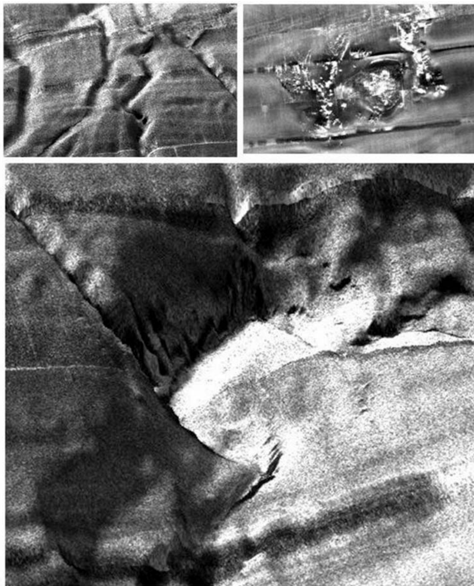
Figure 7.31. Extracts from Figure 7.30. (Top left) 3-D view (sonar imagery draped on multibeam bathymetry) of the Carboneras Fault. Although its 2-D expression is subtle, it can be followed across the entire image, on several swaths, and the offset of tributaries to the main turbidite system strengthen its original interpretation as a fault. (Top right) 2-D view of Chella Bank (see Lo Iacono et al. , 2008 for detailed interpretations). (Bottom) 3-D view (sonar imagery draped on multibeam bathymetry) of one of the meanders in the canyon. Note the deeply incised tributary feeding into it from the northwest, the rougher textures of sediments inside the canyon, and the change in backscatter levels associated with the imaging directions (from the bottom or the top swath).
