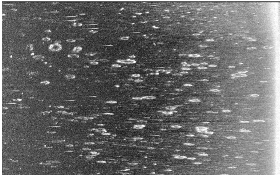
Figure 8.15. High-resolution image of old oyster beds in a shallow lake, acquired with the SwathPlus interferometric, multi-frequency system. The image is 100 m wide and ensonified from the right. Note the across-track distortion of the structures increasing with range, which can be processed using the steps outlined in Chapter 4 (image courtesy SEA Ltd., U.K.).
